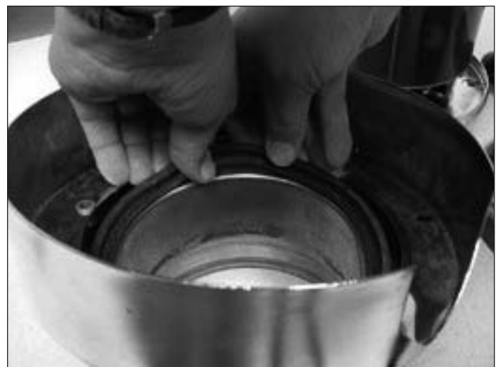
Figure 11. Replacing Shredder Gasket
