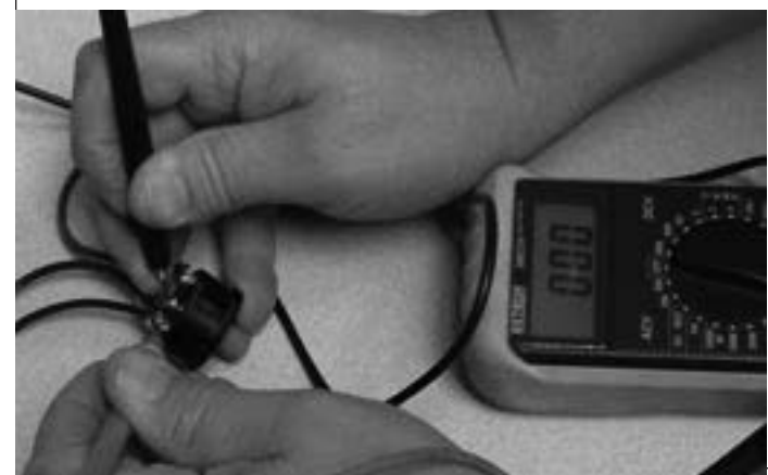
Figure 24. Testing Overload Protector
