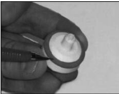
Examining the seal ring on the plunger
