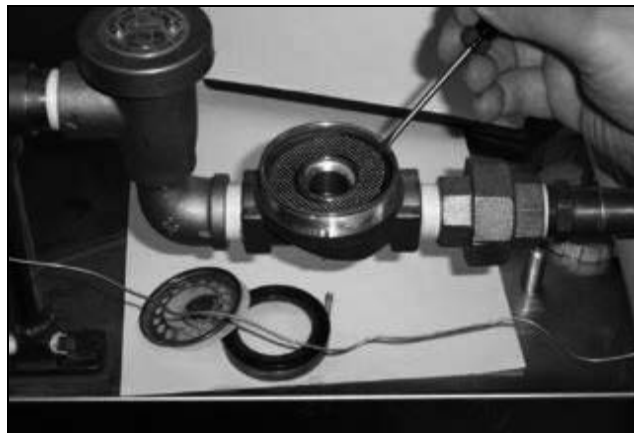
Removing the mesh strainer screen
