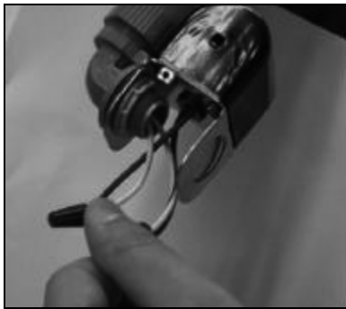
Straightening the wires
