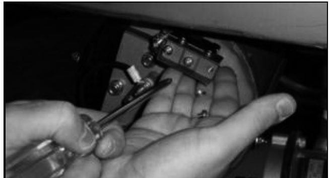
Removing the thermostat screws.
