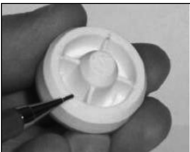
Examining the plunger seating surface
