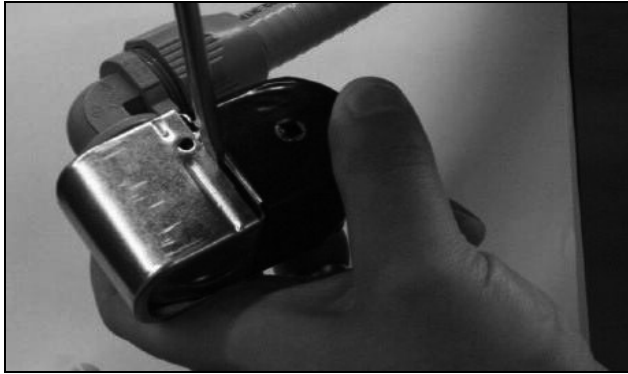
Prying open the coil wire cover
