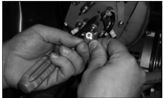
Fitting the jumper into the mounting cup.
