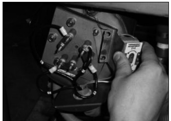
Removing the thermostat bracket.
