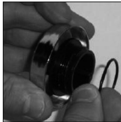
Replacing the O-ring
