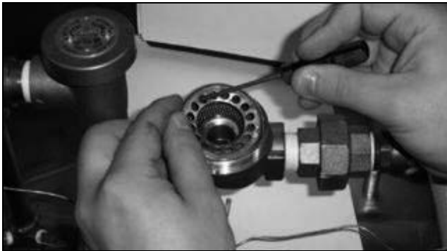
Removing the screen retainer
