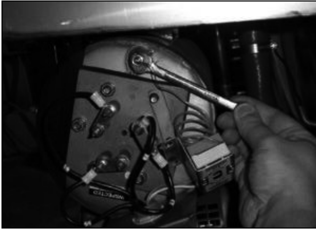
Removing the imperial brass fitting.
