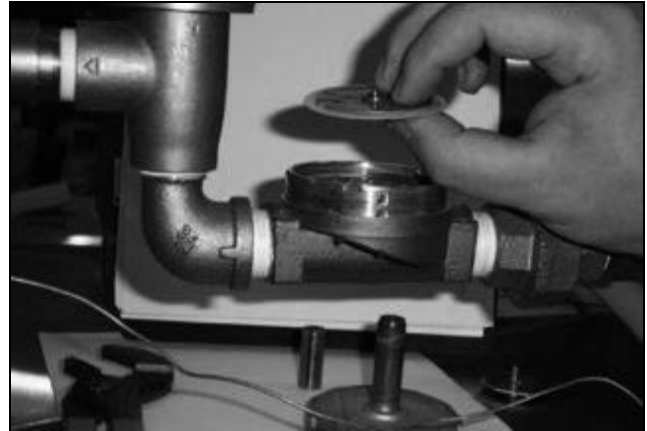
Removing the diaphragm
