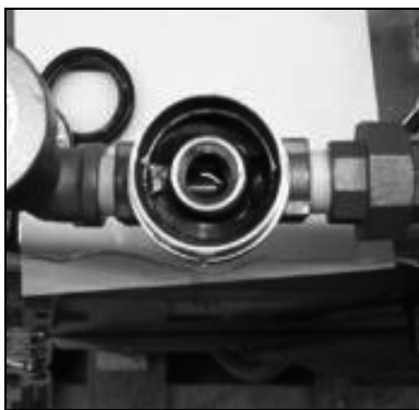
View inside the solenoid valve body
