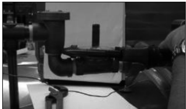
Loosening the valve bonnet
