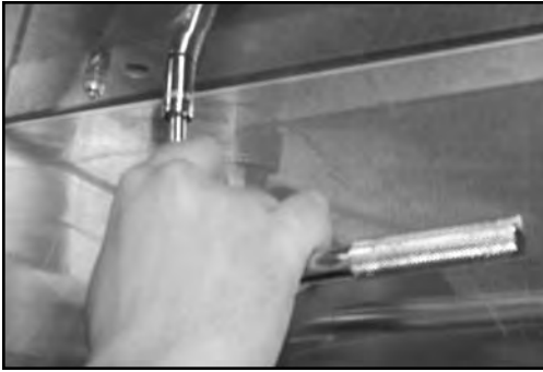
Removing the hole cover weldment
