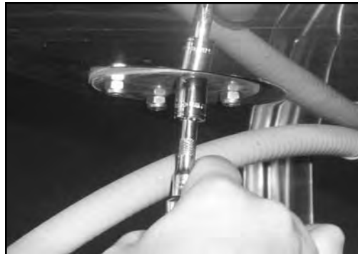
Removing the rinse drain plug
