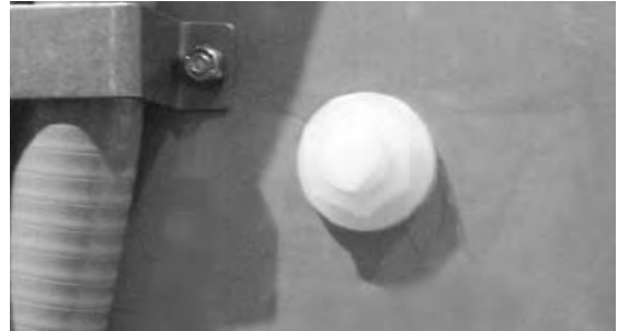
Detergent Connection Point (Machine rear view)
