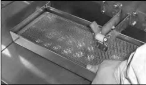
Lifting out the rinse tray assembly
