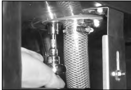
Removing the rinse drain weldment
