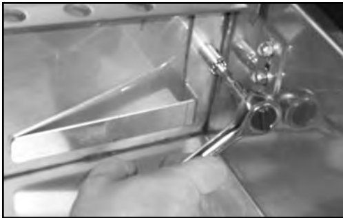
Removing a rinse tray guide bracket
