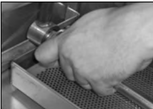
Unscrewing and removing the lower rinse arm
