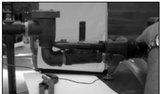
Loosening the valve bonnet
