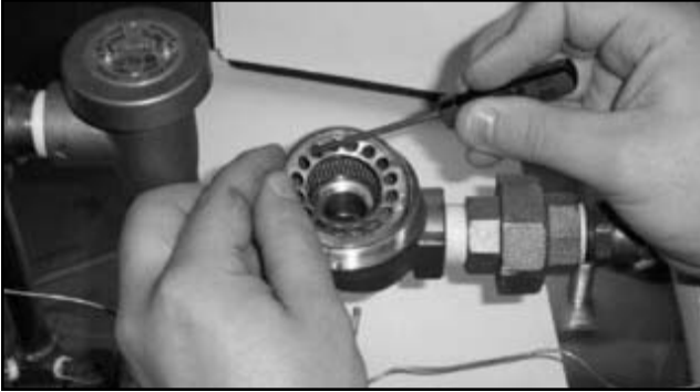
Removing the screen retainer
