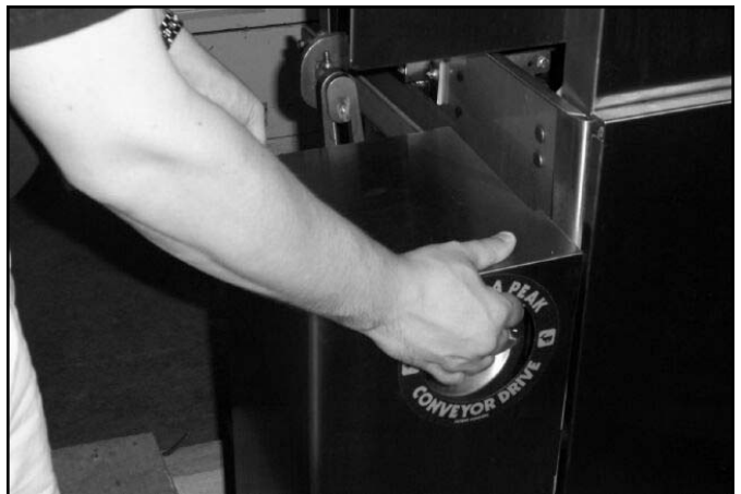
Removing the top cover.
