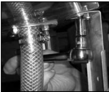
Removing the motor support bracket
