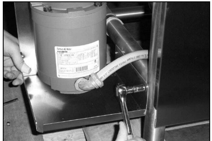
The Correct way to mount the drive motor.
