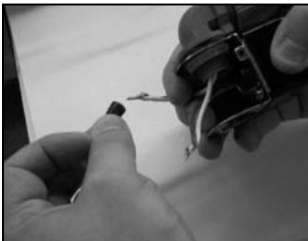
Removing the wire nuts
