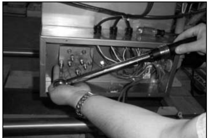
Applying the torque wrench to the nuts
