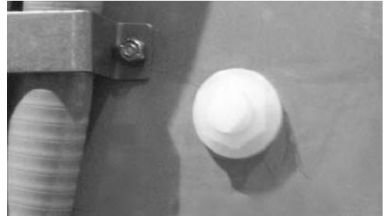
Detergent Connection Point (Machine rear view)
