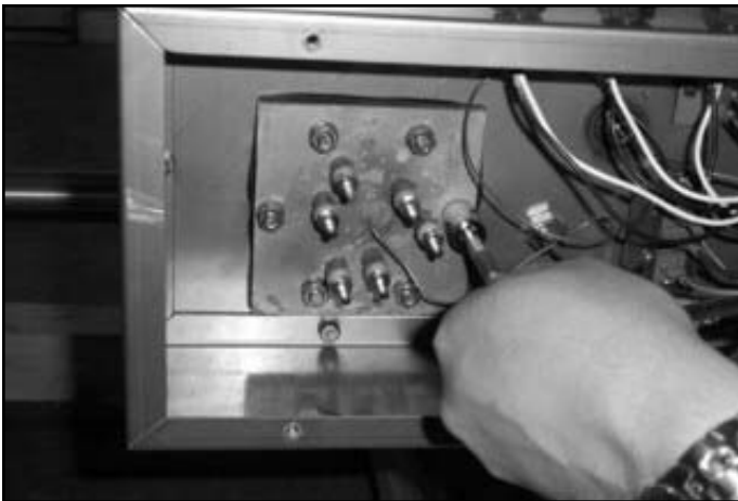
Removing the nuts and lockwashers
