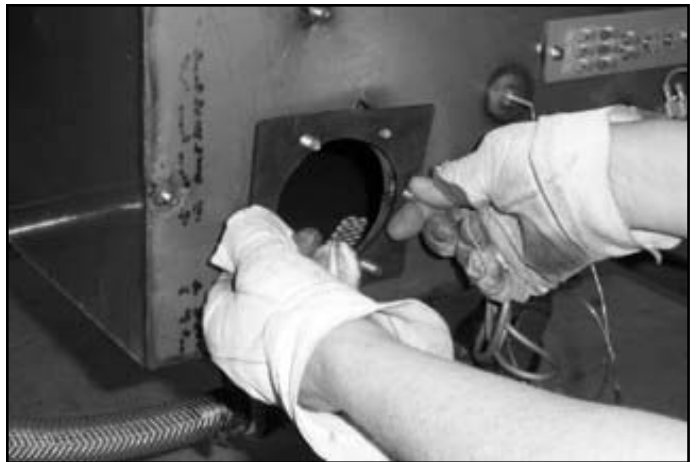
Removing the gasket
