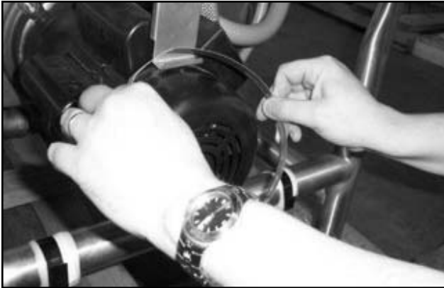
Removing the rear clamp
