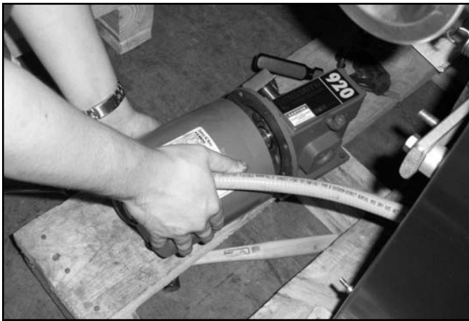
Mounting the motor to the gear reducer.
