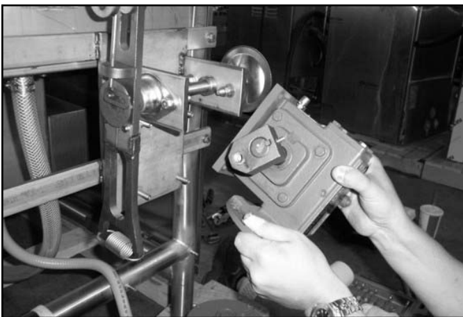
Removing the gear reducer.
