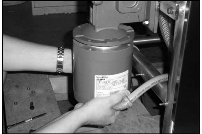
Removing the drive motor.
