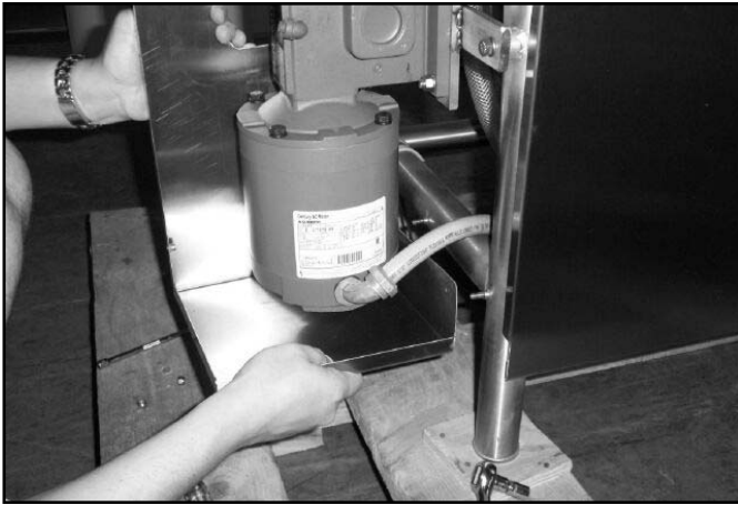
Removing the bottom cover.
