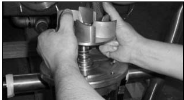
Removing the impeller
