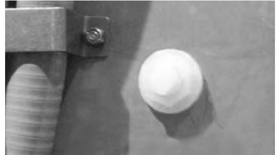
Detergent Connection Point (Machine rear view)
