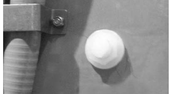
Detergent Connection Point (Machine rear view)
