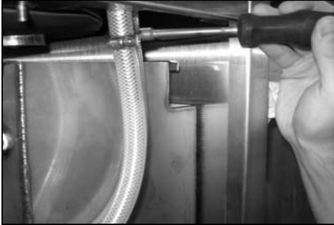
Loosening the discharge hose clamp.
