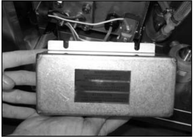
Removing the heater cover.
