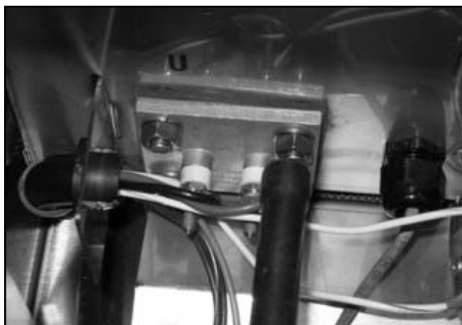
the way. Using the ratchet to remove the heater mounting nuts.
