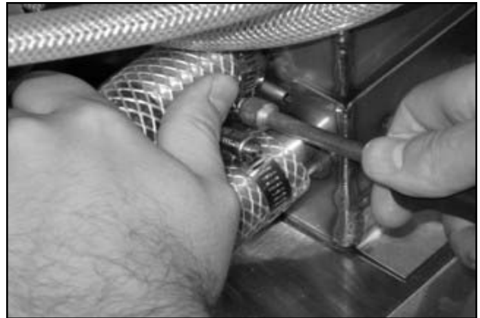
Loosening the suction hose clamps.
