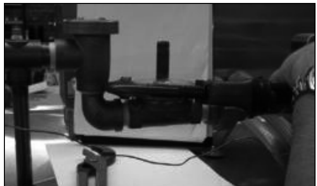
Loosening the valve bonnet
