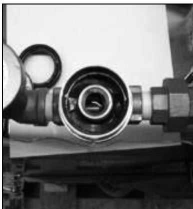
View inside the solenoid valve body
