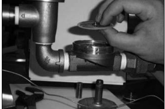
Removing the diaphragm
