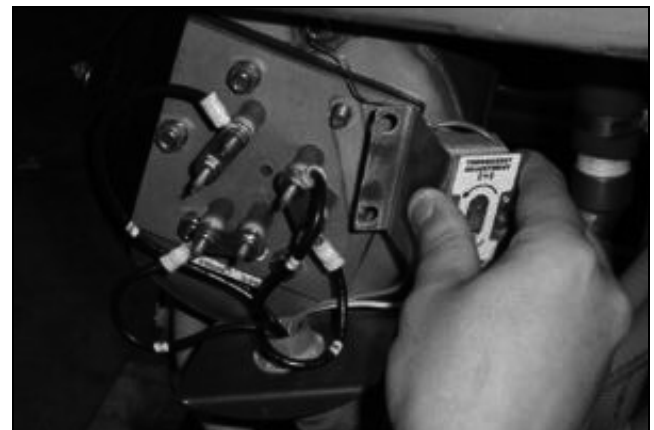
Removing the thermostat bracket.
