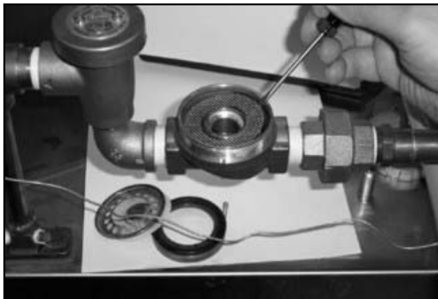
Removing the mesh strainer screen
