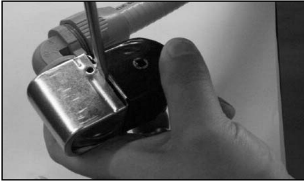
Prying open the coil wire cover
