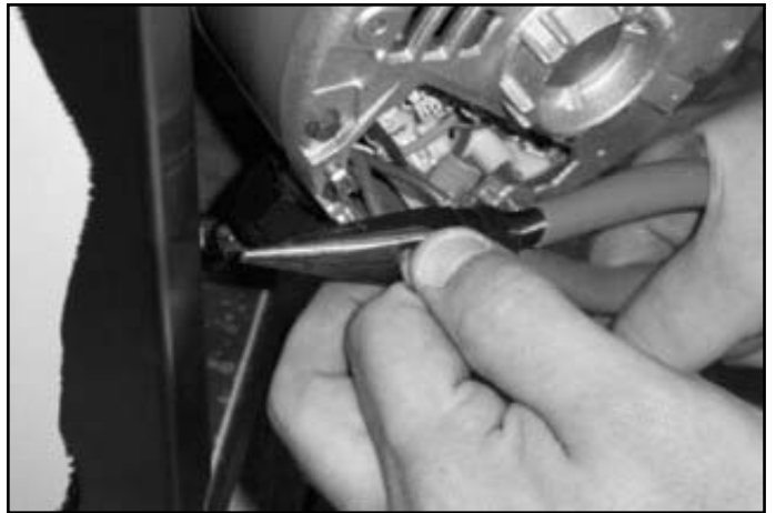
Cutting the terminals off of the power wires.
