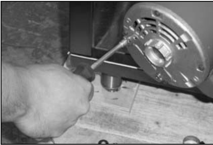
Removing the wiring cover.
