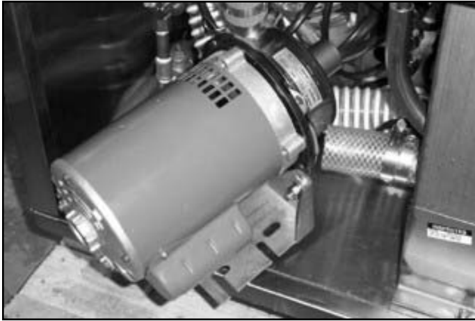
Turn the motor so you can access the rear wiring cover.
