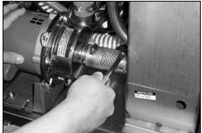
Loosening the suction hose clamps.
