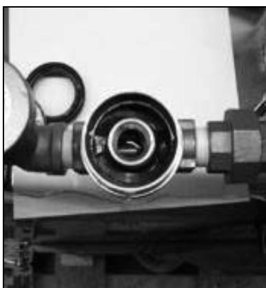
View inside the solenoid valve body
