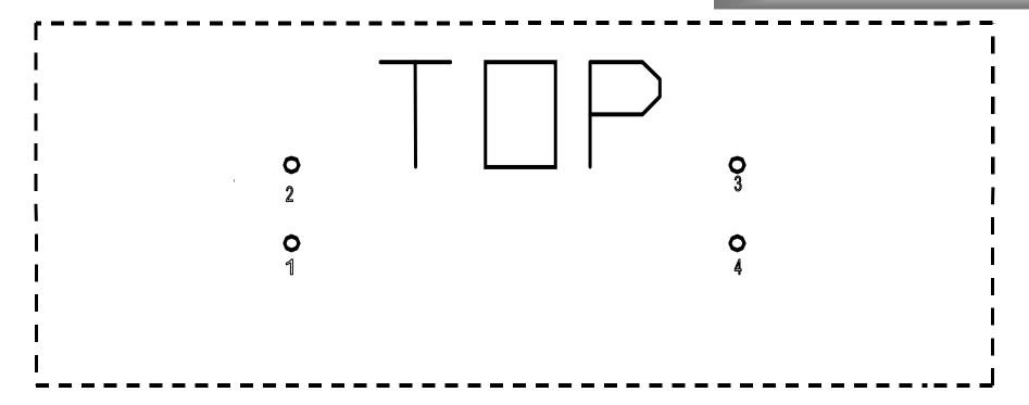
This template is given in the event that the customer would like to install a timer onto the front of the Pane Bella Grill.
