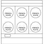
**RF21S-C** Three Hot Tops controlled by three 850° thermostats.
