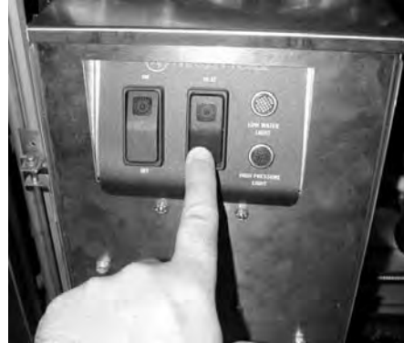
2. Energize heating circuit to pre-heat unit.
