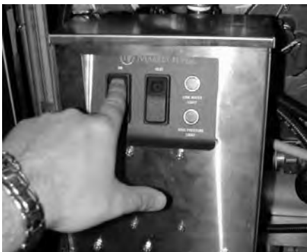
1. Energize boiler and fill to operating level.
