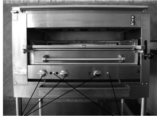
Burner valve knobs
