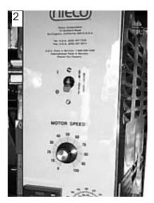
Turn on Motor Power Switch and set Motor Speed Control to desired setting. (Use a setting of "50" to start.)
