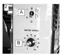
Turn on Motor Power Switch (A) and set Motor Speed Control (B) to desired setting. (Use a setting of "50" to start.)
