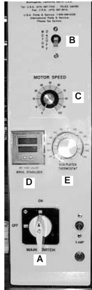
2. Turn on Motor Power Switch (B) and set Motor Speed Control (C) to desired setting. (Use a setting of "50" to start.)
