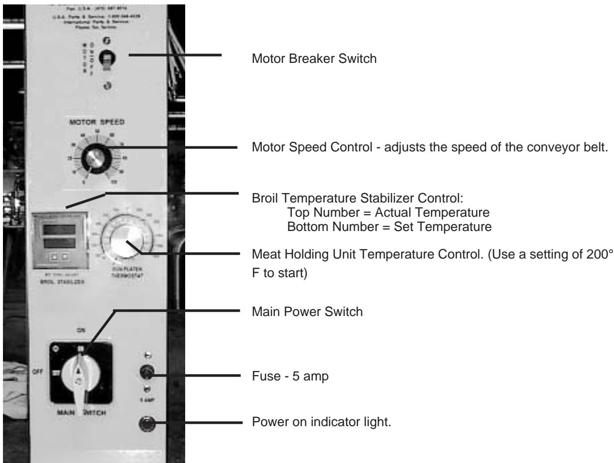
After the hamburgers are cooked, they drop into the Holding Unit, which uses an electrically heated base to maintain a set temperature for holding the hamburgers or chicken.
