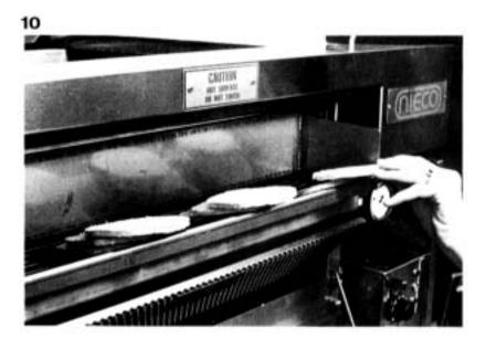
Place the buns directly on the bun belt "cut side" up. Load the tops (crowns) on the right side, and the bottoms (heels) on the left.
