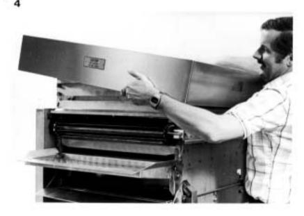
5. Remove GREASE DRAIN CHUTE and GREASE COLLECTOR BOX; clean daily with soap and water.
