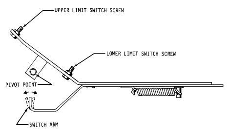
The switch trip mechanism is binding. (Clean the mechanism and lubricate its pivot point, see above illustration.)
