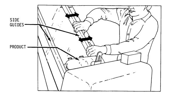
Adjusting the Outfeed Side Guides on a Standard Outfeed Table
