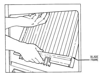
Removal of the infeed side blade frame is accomplished in a similar fashion. However the chute guard must first be removed by removing the four knobs which hold it in place this will allow access to the locking cams. See the illustration below.
