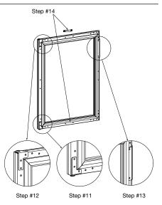
STEP 11 to bracket. Re-assemble door hinge bracket to previous position with bushing attached.
