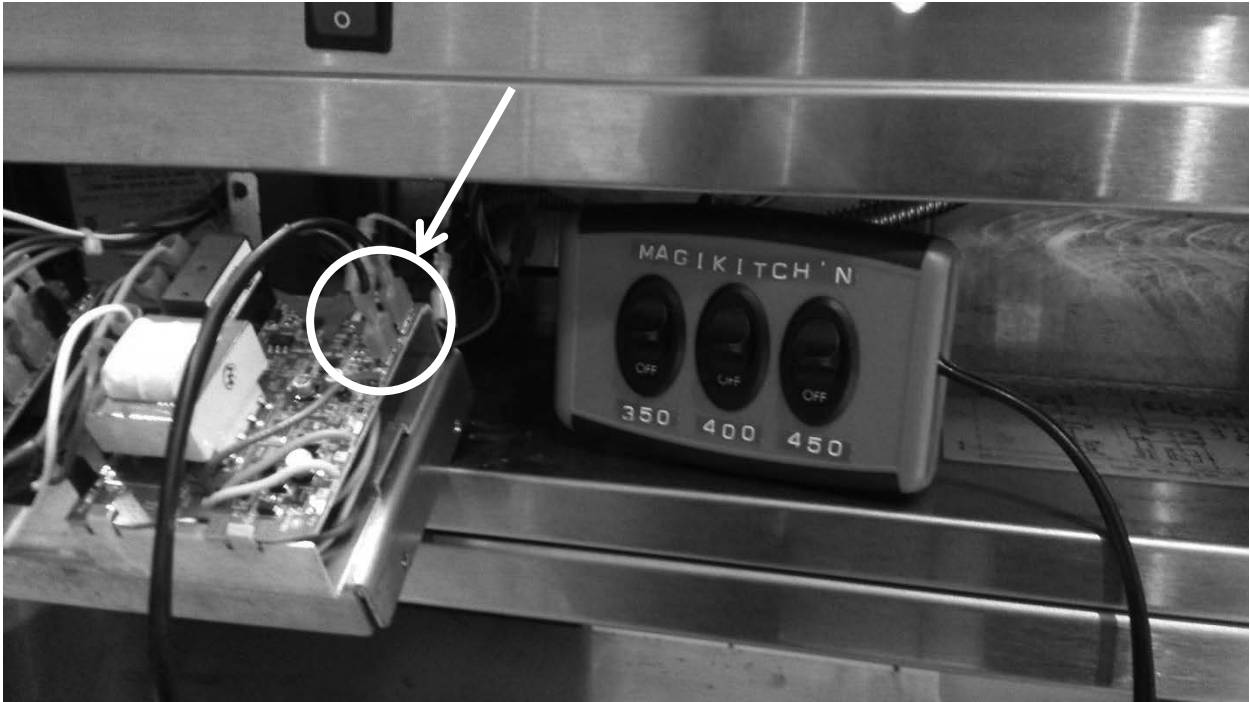
Figure 9: Unplug the T-Stat wires from the first controller and replace it with the leads from the Calibration test tool, as shown above (leads do not have to be in any certain order/position).
