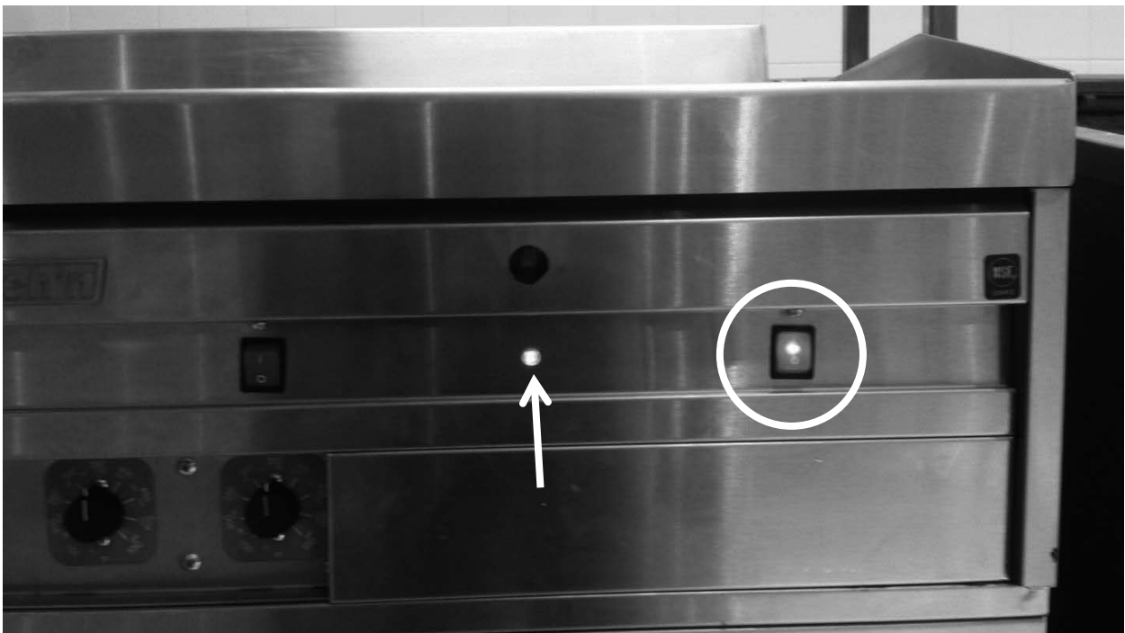
Figure 2: To validate that the unit is operational, turn on one set of burners by pushing the button (circled above). Pilot should light and indicator light should illuminate (indicated by the arrow).
