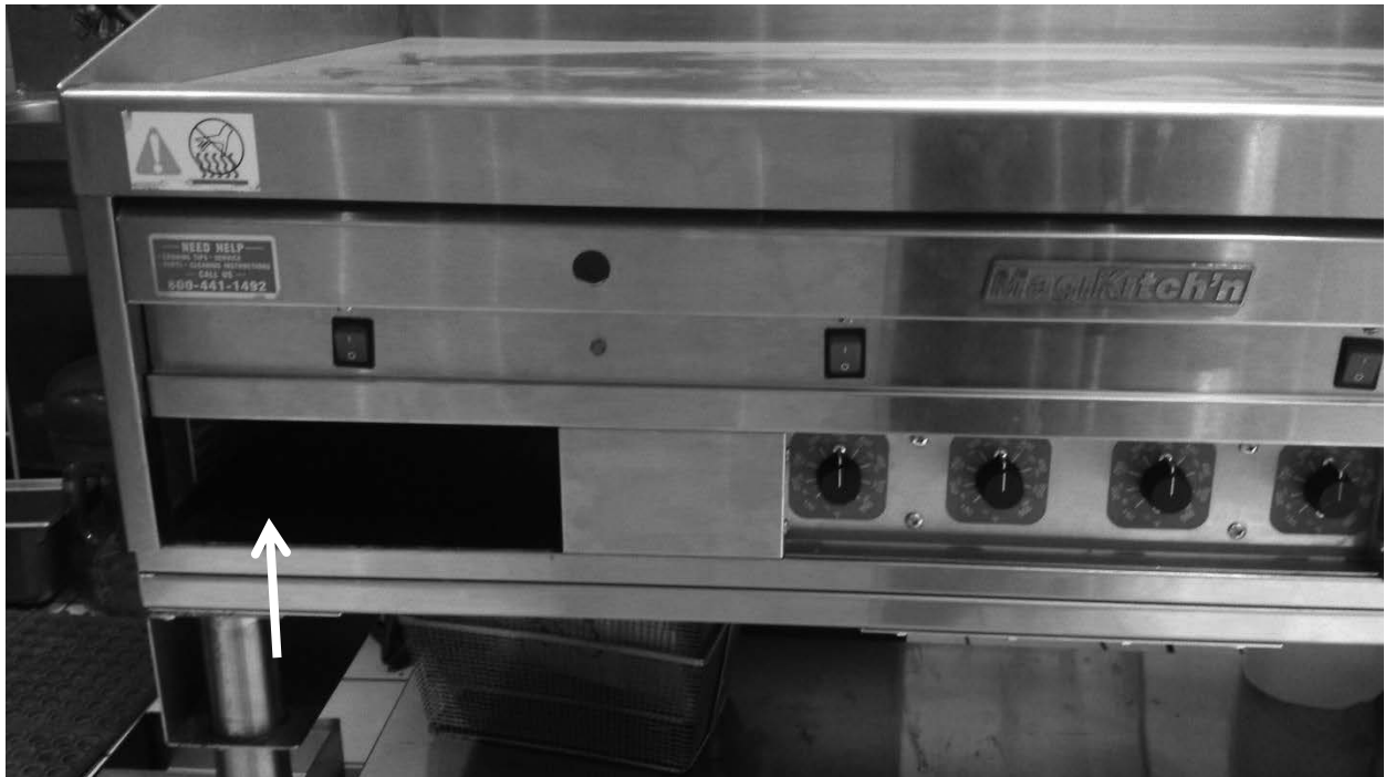
Figure 3: To gain proper access to the Thermostat wires, some disassembly of the unit is required. Start by removing the grease pan, indicated above.
