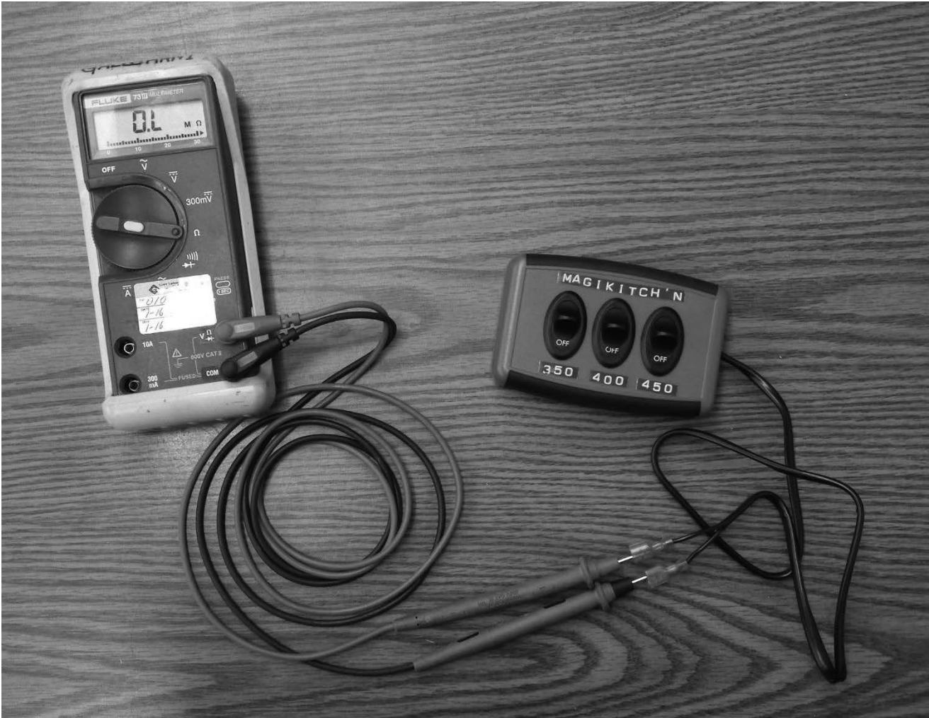
Figure 15: To verify the calibration device, connect your multi meter/ohm reader as shown above.
