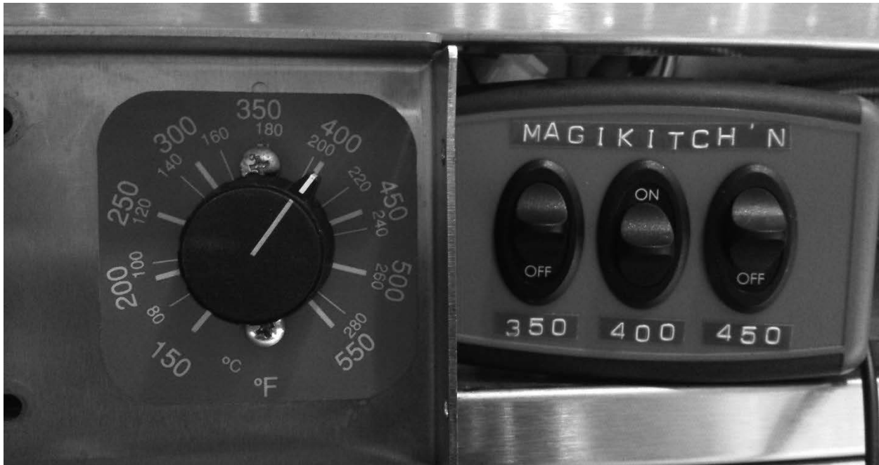
Figure 13: Once the control knob is in the correct spot, using the Calibration tool, verify that the control knob works in the other two temperature locations.
