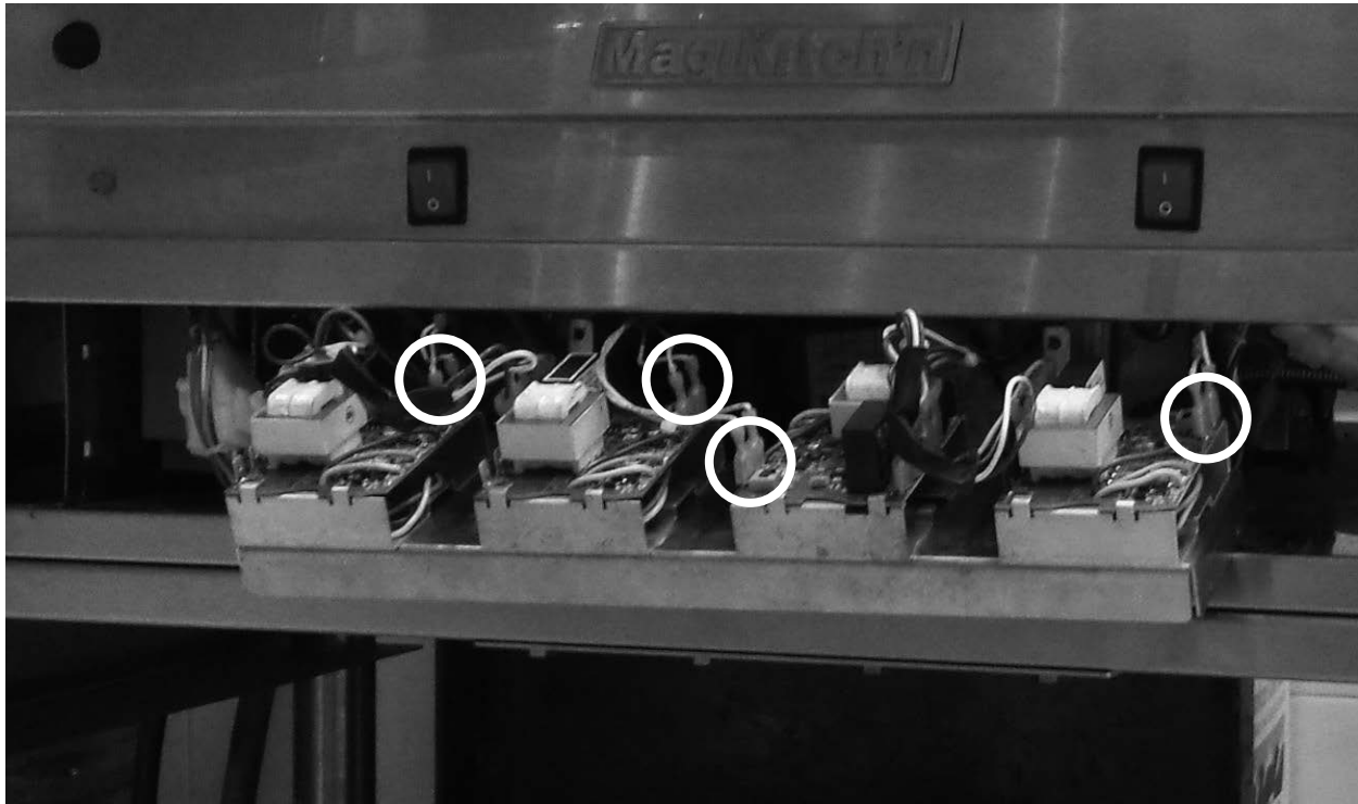
Figure 14: Repeat all of the above steps for each of the Solid State Thermostat controls. Making sure to re-install the units Thermostat plugs when complete with each controller (Thermostat wires do not have to be in any particular order/position).
