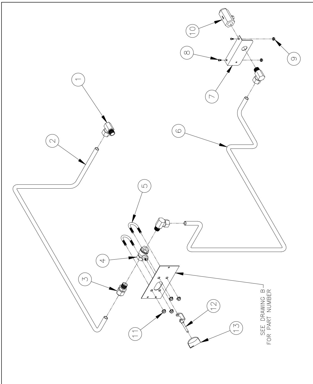
**I) Mixing Valve Option****Mixing Valve Option Drawing I Parts List**
