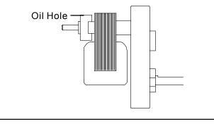
The conveyor chain should not touch the top surface of the crumb tray holder. If the chain does touch, retention it by unplugging the unit, remove both side covers, loosen the front bearing mounting screws and pivot the bearing until the chain no longer touches. Retighten bearing screws and replace side covers
