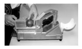
Push handle with a quick, firm stroke all the way through the blades and until the pusher stops.
