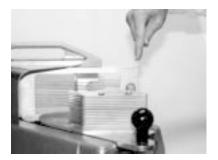
3. Slide in the new blade cartridge with arrow facing up. See figure 6.
