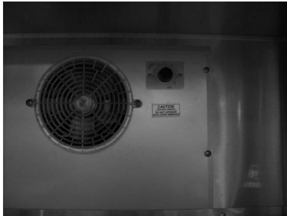
Figure 1 illustrates the evaporator fan shroud assembly. The thermostat adjustment knob for the display merchandiser is located on the top right of the evaporator fan shroud. Access to this area can be obtained by removing the doors, shelving, and mirror.
