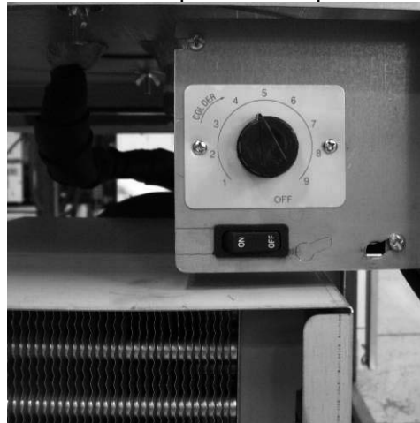
Figure 1 illustrates the electrical control box inside the mechanical compartment. The thermostat adjustment knob for the refrigerated rail is located on the top portion of the control box.
