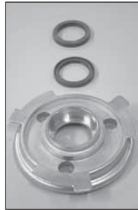
8) Replace shaft seals
