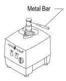
5. Turn the blade cap clockwise to tighten or counterclockwise to loosen. The bottom blade should hit the stop on the blade tool and prevent the assembly from turning. Do not overtighten.
