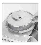
Next fit the appropriate slicing disc and rotate in a clockwise direction to check that it i correctly positioned.
