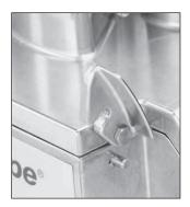
3) Position the head of the vegetable preparation machine on the motor shaft. The fastening hook should now be facing you, on your right.
