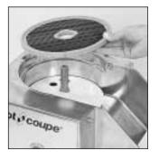
Make sure the plastic tab on the outer rim of the grid is fully seated in the corresponding slot in the motor unit.
