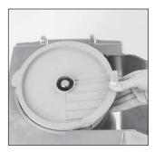
Next put the appropriate slicing plate on the motor shaft.
