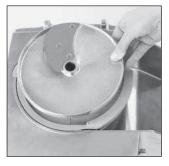
Rotate the plate until the slot in the plate hub falls over the motor shaft pin. Continue to rotate one full turn. If the cutting plate scrubs the grid-do not proceed-call your authorized service agency.
