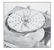
3) Always have the hollowing nut in place when you are not using the divider. Screw the hollowing nut down over the plate, and into the motor shaft.
