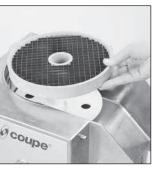
Make sure the plastic tab on the outer rim of the grid is fully seated in the corresponding slot in the motor unit.
