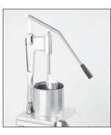
4) Position the large lead assembly on the motor base. The latch is now facing you on your right.
