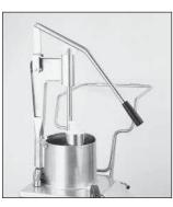
The plates can be changed without dismantling the feeding tray.
