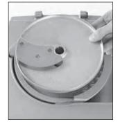
Next fit the appropriate slicing disc and rotate in a clockwise direction to check that it i correctly positioned.
