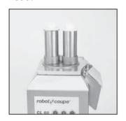
3) Position one or the other of the tube feed heads on the motor base, with the fastening hook facing you, on your right.
