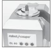
3) Screw the rubber agitator onto the motor shaft.
