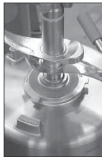
12) Push down blade assy, stop when hits motor shaft
