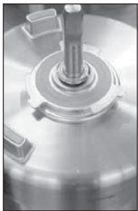
10) Replace shaft top seal, place it on shaft chamfer
