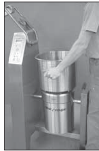
14) Attach the bowl with the pouring lip on the left hand side.
