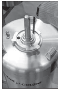
5) Remove bolts and washers
