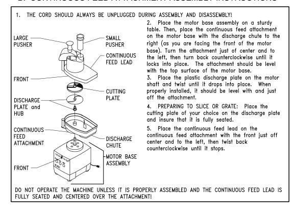
The continuous feed lead serves several functions. Primarily, the lead protects the operator from the cutting plate. When the lead is fully locked in place, the plate is covered and the unit will be ready for operation.
