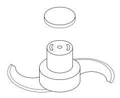
There is a removable cap attached to the top of the S-blade assembly. This cap should be removed when cleaning the blade assembly.
