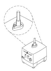
Put the blade on the blade-stop, and insert the metal rod into the hole near the top of the blade assembly. Then, turn the blade assembly counterclockwise until it contacts the raised tab on the blade stop. The blade assembly will come to a stop when it hits the tab on the blade-stop. At this point, continue to turn the rod in the counterclockwise direction, until the top locking nut releases and unscrews.
