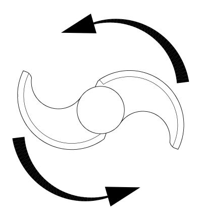
Three phase motors may rotate either direction.
