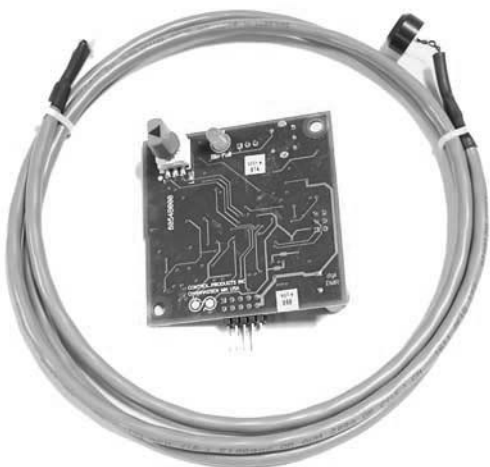
Ultrasonic Board and Cable
