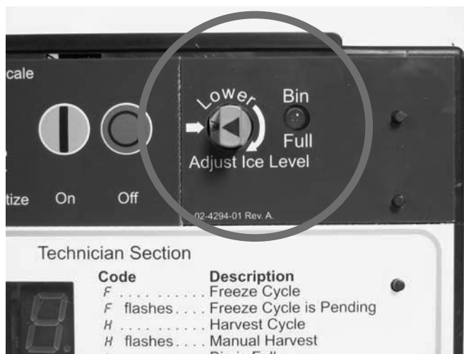
Ultrasonic control shown in its installed position, set at maximum fill.
