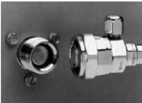
Clean and Lubricate Couplings
