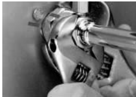
Rotate Swivel Nut \frac{1}{4} Turn More
