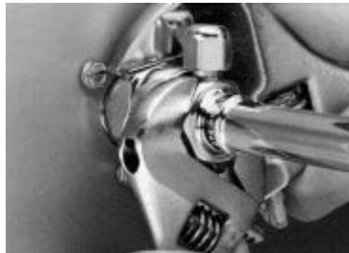
Tighten Swivel Nut
