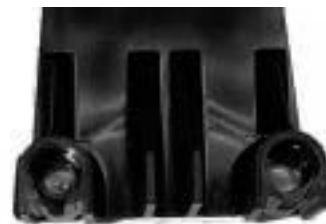
Lens Location in Ice Sensor
