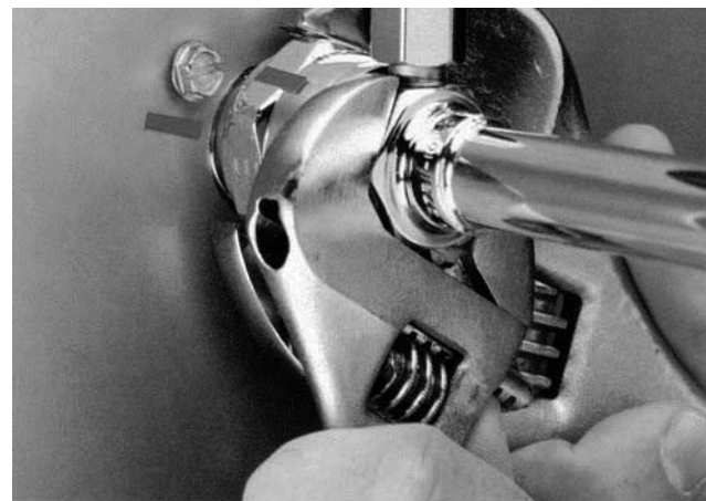
Rotate Swivel Nut ¼ Turn More
