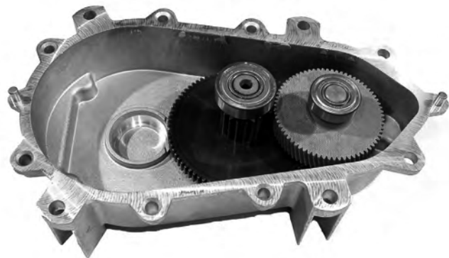
Gear case with First and Second Gears
