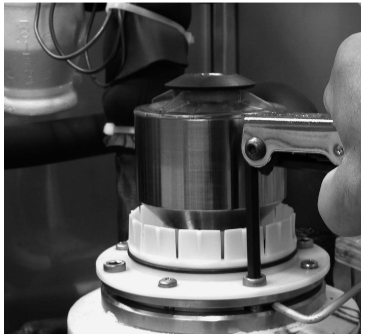
Remove allen head cap screws
